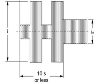
(4) Motor Load  $i/i_o = 5$  to 10 times
