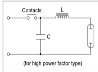
In general, discharge lamp circuits use a combination of a discharge tube, transformer, choke coils, and capacitors. Note that the lamp may draw an inrush current may be 20 to 40 times the steady-state current, especially if the supply impedance is low in the high power factor type.
