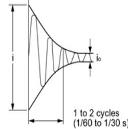
(7) Capacitive Load  $i/i_o = 20$  to 40 times
