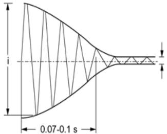
(6) Electromagnetic Contact Load  $i/i_o = 3$  to 10 times
