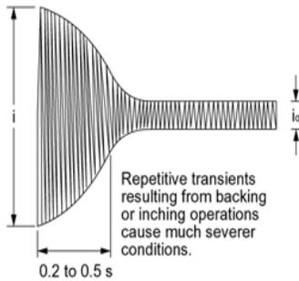
(5) Solenoid Load  $i/i_o = 10$  to 20 times
