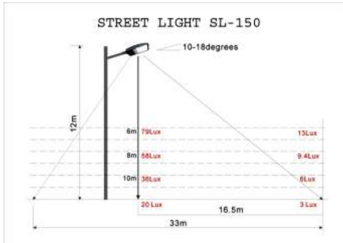
Typical Intensity Pattern of 150W street Light
